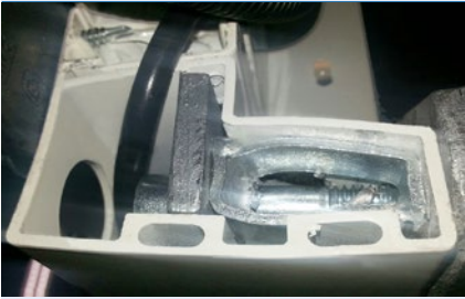
tightening torque too high
