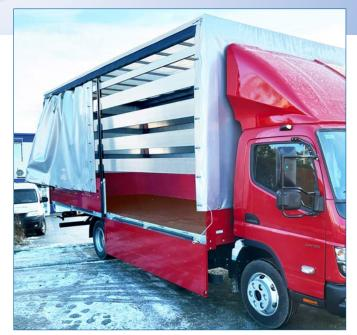
Alternatively, you can also obtain the tried-and-tested **GRP fixed roof** for the box body kits. In addition to the lower price compared to the sliding roof, it is advantageous that the roof allows light to enter the loading area. The smooth roof skin also prevents water from collecting (water pockets), which significantly reduces the risk of ice sheets forming.
